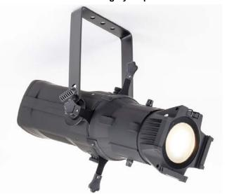
The Elektralite Stingray is a 300 watt LED ellipsoidal with the output of a conventional 750 watt fixture. Different LED types are available including Warm White, Cool white, RGBA, and 7 color. Lens available are 19°, 26°, 36°, 50°. Special Lens also available : 5° and 10°. The Stingray will accept other manufacturer's lens as well as Elektralite's own lenses.
